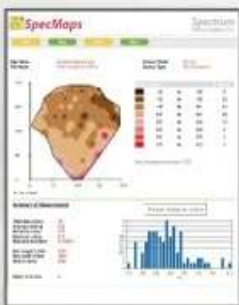
SC 900 on a baseball field: Yellow and red spots indicate areas of heavier soil compaction.
