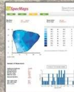
TDR 300 on a putting green: The areas with higher soil moisture are shown in deep blue.
